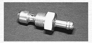
Place a hose clamp over the end of one hose. Push the hose end over oil pan outlet
