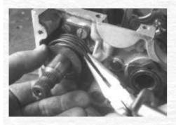
The kick-starter mechanism also needs re-fitting before the cases can be joined. It slots in behind the gear selectors and is then retained by a catch plate and circlip. Here I'm tensioning up the return spring and hooking it in. Make sure the kick-starter is fitted correctly before proceeding, it's hard to think of anything more frustrating than to discover it doesn't work once the engine is back in the bike !
