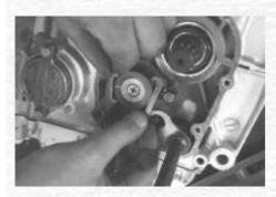
On the drive side of the engine now, I'm hooking the gear selector claw into place before re-fitting the mission cover with a new gasket and oil seals. Note the circular cover forward of the mission cover which covers the left hand end of the jackshaft. This is a good opportunity to check the gear change mechanism by selecting up and down through the gearbox. If any problems show up sort them out now before carrying on with the rebuild.
