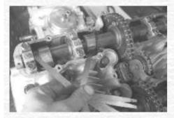
As I've re-faced the valves and seats the shim clearances now need to be checked. Correct clearances are 0.10 - 0.15mm at the widest point but as with all DOHC engines these clearances will tend to reduce rather than increase, and it is vital for the health of the valves that some clearance is present. I'm going to recommend another shim check after the first 500 miles as the valves will tend to bed in.
