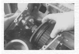
The jackshaft now slots into the crankcase from the clutch side. The primary chain has to be engaged on its drive sprocket on the shock absorber assembly and the starter clutch has to be in place before the jackshaft will slide home. A little fiddly, but not quite as complex as it may look. Finally the roller bearing on the end of the jackshaft has to be tapped into place in the crankcase; I use a socket big enough to bear on the bearings outer race to avoid damaging the bearing.
