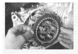
The clutch plates were badly worn too, so I'm fitting a new set of friction plates. To prevent the plates sticking together I've oiled each new clutch plate before fitting it. A new set of clutch springs finishes the job off.
