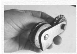
Early Z650s used a combination of sprockets and rubber idler wheels to guide the cam chain run, later replaced in favour of simpler slipper blades. This is the main guide roller assembly which fits at the rear of the barrel and is pivoted by the cam chain tensioner. The rubber roller has hardened with age and worn dimples around its working face, and I'll be fitting a new one. However this may not be a cheap option.
