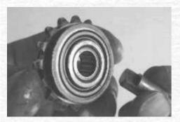
And this is one of the cam chain guide sprockets. These are supported in tiny needle roller bearings and it's as well to check to make sure the rollers are intact, as they are here. Note the flats on the end of the bearing pin - these are sandwiched against tiny rubber blocks between the head and barrel which also harden with age. Nothing wrong with the sprocket, but I'll be replacing all the tiny rubber blocks.
