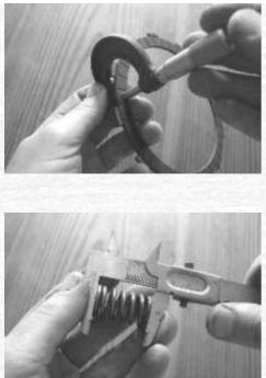
The clutch plates look a little on the thin side. Sure enough when measured they're under the service limit of 3.5mm, and I'll be fitting a new set for the rebuild. Only the friction plates need replacing, the plain plates will have only suffered if they've buckled due to very hard use or racing. Check the plain plates on a flat surface to make sure of course, but under normal use they should last more or less indefinitely.
