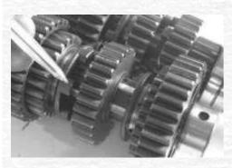
Check the individual gears for chipped or broken teeth, or worn or damaged dogs here. The selector forks which engage in the sliding gears should also be checked for any damage or wear and particularly bent ends if any selection problems have been encountered. Bent or damaged selector forks should be replaced with new ones - don't try to straighten them.
