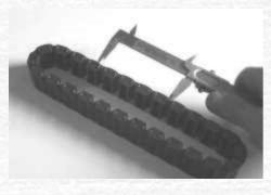
The primary chain is an enormous Hy-Vo device, massively strong but also massively expensive to replace. Kawasaki advise measuring wear by looking for sideways play which should not exceed 27mm, which you can do with the sump removed and the engine in the bike. Here I'm checking for length between the pins. There's no tensioner provided for the primary chain. I'm not surprised, to find this one is well within its service limit.
