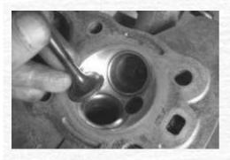
With the buckets lifted out the valves all release with a conventional valve spring compressor, though the limited space around the valve top collar means some compressors sold for car engines will not fit. There is some carbon build up on both the combustion chambers and valves, but both clean off fairly easily. The valve seats themselves look in surprisingly good condition, with only very light pitting on the sealing faces.
