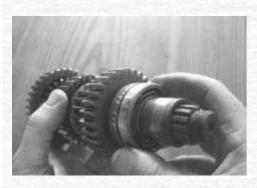
Next in the pile is the gearbox shafts and gears. The Z650 has a strong transmission design and rarely gives problems here, but its always worth checking while its apart. This bearing on the output shaft fits behind the engine sprocket. If the rear chain has been run too tightly it will have put too much load on this bearing. If any signs of wear replace it now, and use a genuine bearing rather than one from a supply shop.
