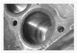
Moving up the engine it's time to take a good look at the cylinder bores. There is some sign of surface corrosion, particularly on No.2 (shown) but as this isn't deep it may not be too much of a problem. I'll be honing out the bores before rebuilding the engine, and as long as the bores are within tolerance afterwards it will be fine. Deep pitting would mean a re-bore.
