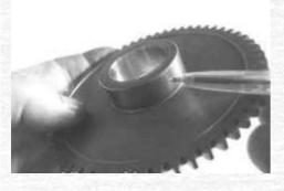
This is the boss on the drive gear which should wedge against the rollers in the starter clutch. Any sign of flatting, or "three-penny bitting" on the boss means the starter clutch can slip under load. This one has the first signs of wear and is approaching the end of its service life. Replacing it now may not be the cheap option but it may save another engine strip to change it in a few thousand miles.
