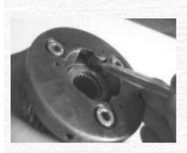
The starter clutch follows conventional Japanese design. These three rollers are fitted in wedge-shaped slots, and held outwards by small springs and plungers. When the starter is engaged the three rollers are wedged against the drive gear to transmit the drive. After high mileages the three rollers can begin to develop flats and may not lock against the drive gear correctly, making the starter spin without turning the engine over. Now is the time to fit new rollers and springs.
