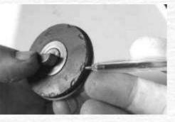
This rubber guide wheel, also from the cam chain, is showing signs of breaking up around the working edge. It's also become quite hardened and brittle compared to a new one, so it goes on the list for replacement too.
