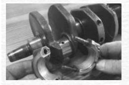
Unbolting the big ends from the crank reveals the old bearing shells. I always replace shell bearings as a matter of course, but the condition of the old shells can give a good indication of the state of the crank itself. These shells are showing typical signs of wear but no undue scuffing, and the big end journals look smooth and polished. The micrometer confirms they're still within factory tolerances.
