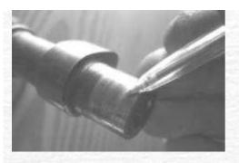
Moving higher up the engine the first sign of a potential problem is found. On this Z650 the cam bearings are machined straight into the head, which means the cams run direct in alloy. The integrity of the cam bearings therefore depends on a constant supply of clean oil and if oil changes are missed or foreign bodies allowed to enter the engine these bearings will suffer first. Some of the cam bearing journals are showing signs of scoring.
